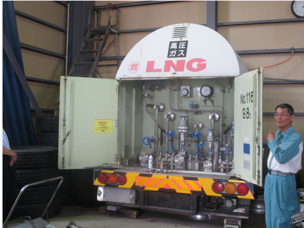
Photo 3: Simulator for training truck drivers in loading and unloading operations for LNG from containers and trucks. Photo by Richard D. Stewart
