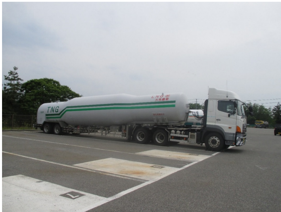
Photo 2: LNG 15 metric ton Bulk Tank Truck. Photo by Richard D. Stewart
